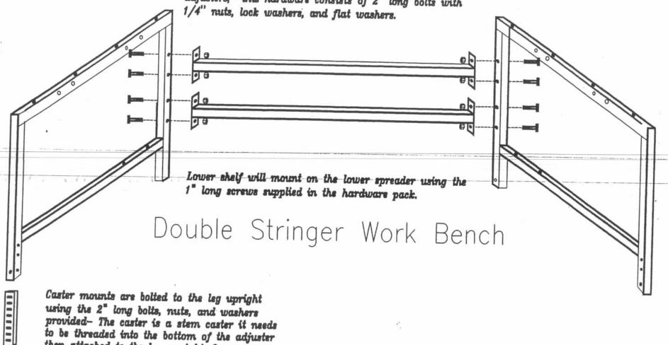
Caster mounts are bolted to the leg upright using the 2" long bolts, nuts, and washers provided- The caster is a stem caster it needs to be threaded into the bottom of the adjuster then attached to the leg upright. On a non-adjustable Ht. bench, the caster screws directly into the bottom of the leg where a threaded part will be welded in place.
